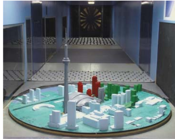
Fig. 3. Wind tunnel testing in an urban setting
